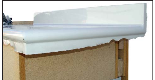
Untrimmed deck casting is positioned on trim table.
