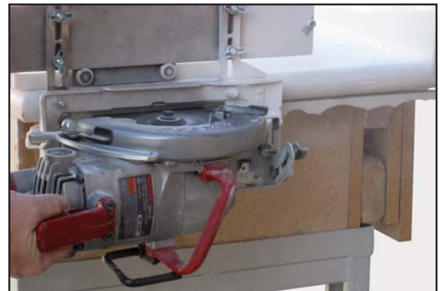
The saw is pulled towards the operator to trim the excess material.
